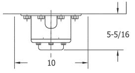
HORIZONTAL KEYWAY:  $3/4 \times 3/8$  VERTICAL KEYWAY:  $1\ 1/2\ \times 3/4$  NORMAL ROTATION: BOTH SHAFTS CLOCKWISE
